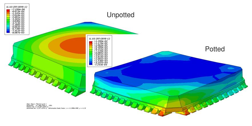
Order of magnitude higher deformation and deformation concentrated over corner solder joints
